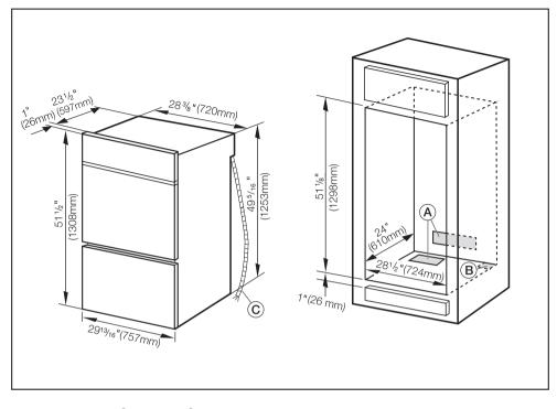
A Vent (min. 24"<sup>2</sup> / 150 cm<sup>2</sup>) cut-out possible at rear or platform of cabinet
